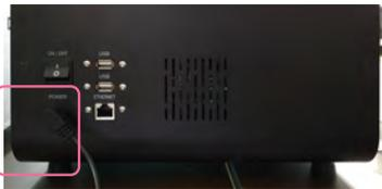
② Turn on the power switch at the back of the 3D printer.
